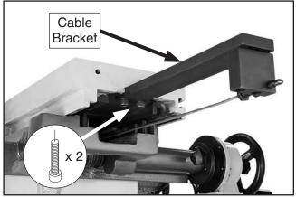
Figure 20. Cable bracket installed.
